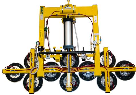
To reduce the risk of load damage, this Powr-Grip® vacuum lifter provides effortless power tilting and optimal support of stone and other high-density materials.
